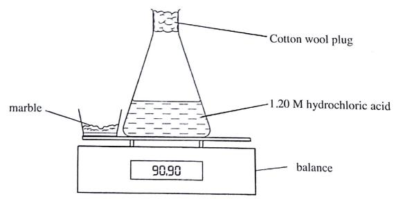
The marble was added to the acid and the mass was recorded every 30 seconds. The experiment was repeated using the same mass of marble but finely powdered. The volume and concentration of the hydrochloric acid were the same. The results of the two experiments were recorded as shown in Table 3.
